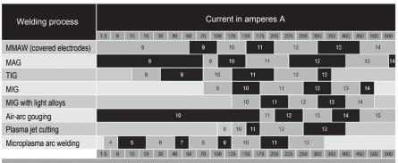
The table recommends best dark shade of welding filter for various working applications. According to the conditions of use, the next greater or the next smaller scale number can be used.
